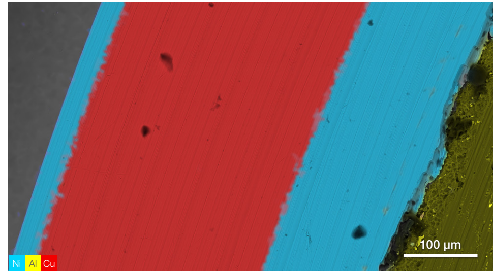
Copper and nickel-coated aluminum alloy. As Cu and Ni have similar atomic numbers, the compositional contrast is not enough to clarify where a coating ends and where the next begins. The Axia ChemiSEM image provides such information within seconds. Acc voltage 20 keV, beam current 3.6 nA.
